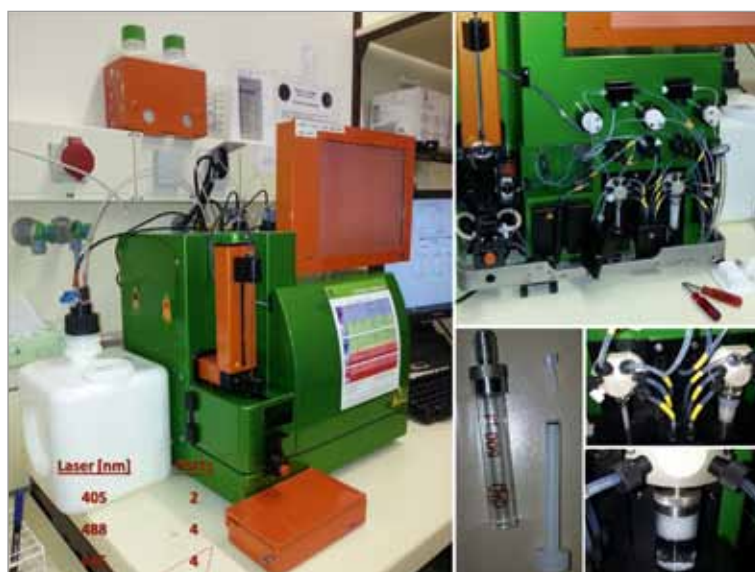
Figure 1. MACSQuant Analyzer 10 (3 lasers, 8 fluorescence channels). Part of the repair and maintenance is carried out by members of the Fluorescence Cytometry staff. The in-depth technical knowledge also leads to improvements of the equipment (e.g. the custom-made attachment of high capacity fluid containers for usage with 96-well plates).
