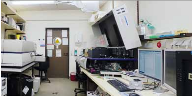
Figure 2. Two high-end analyzers BD LSR II - The multicolor "flagship", which has been upgraded with its new detectors. It can now analyze up to 18 fluorescence channels in parallel. An additional used BD LSR II was acquired and upgraded to provide an identical backup system.
